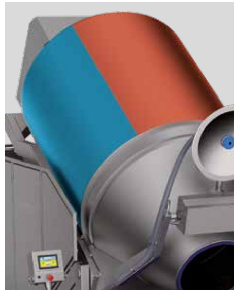
Refrigerated-heated jacketing with automatic thermal control
