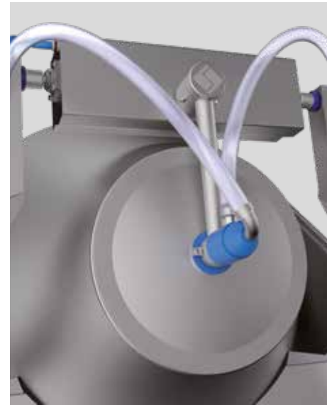
Automatic brine loading system
