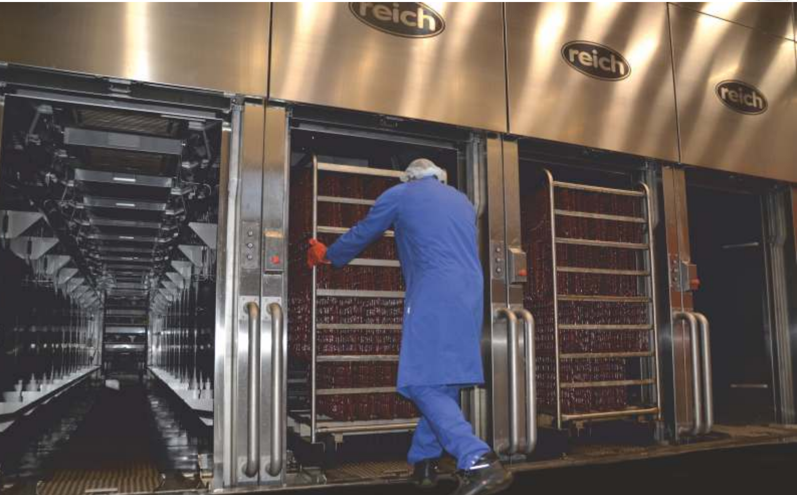
Industrial plant in the Netherlands (8 x UK 27500 BHD for 11 trolleys each with automatic lifting gates)
